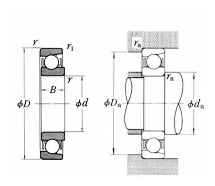
The inner groove of NSK magneto bearings is a little shallower than that of deep groove bearings. Since the outer ring has a shoulder on only one side, the outer ring may be removed. This is often advantageous for mounting.
